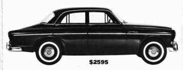
You install 15-inch wheels because big wheels go around fewer times to get you where you're going. The fewer revolutions the wheels make, the fewer revolutions the engine makes and the longer it lasts. Tires last longer, too, and give you better traction in mud and snow.
