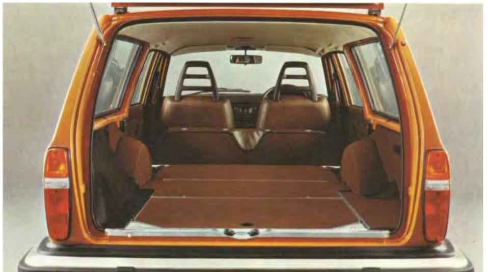
*Just folding down the rear seat increases the cargo capacity from 53 cubic feet to almost 67 cubic feet. The tailgate opening is 45.7" wide and 30.7" high - room enough for a six-foot settee. A pressurized spring makes the tailgate easy to open and it is held up by means of a self-locking mechanism.*
