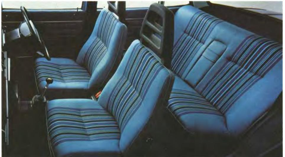
*Volvo's new seats have integral type head restraints. The driving seat height is now instantly adjustable by means of levers.*
