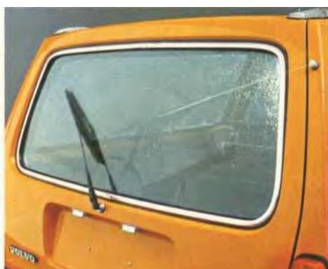
*Seeing behind you is just as important as seeing ahead. Which is why the tailgate window of the Volvo 245 DL is heated electrically and has a wiper and washer.*
